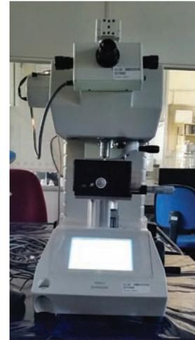
**Fig. 4:** Microhardness tester
