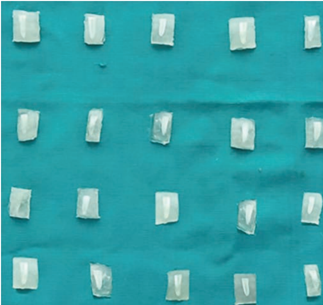
Fig. 4: Specimens embedded in acrylic resin blocks
