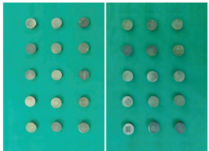
Fig. 1: Samples of laser-sintered Co-Cr disks
